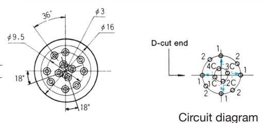
●The circuit diagrams show the switches as viewed from the terminal side with the shaft fully turned in the counter-clockwise direction.
