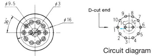
※Two Common terminals (1C) are internally short-circuited. Select either one depending on wiring arrangements.
